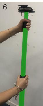
7. Rotate the upper locking sleeve to the right to loosen it, and place the upper telescopic tube to the desired length, adjustable up to a maximum of 28cm
