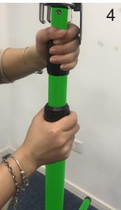
5. Set the middle telescopic tube to the desired length, adjustable up to a maximum of 32.5cm
